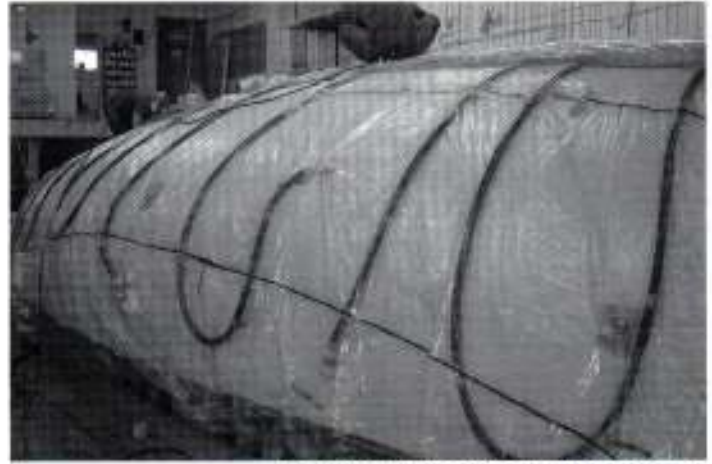
Vacuum bagging a 65' boat at Covey Island Boat works
